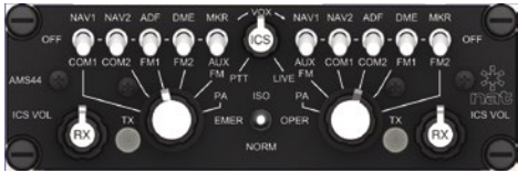
AMS42/AMS42F/AMS44 Flexible design for installation on VFR, OAS, forestry, charter, corporate, fleet, IFR, and police platforms. Features Com, Aux, FM and PA transceivers, RX- and ICS-level controls for each side, and three (3) ICS modes: LIVE/KEYED/VOX.
