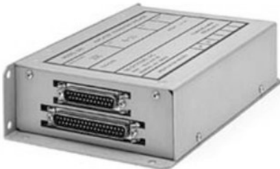
240 Passenger speaker amplifier providing Fasten Seat Belt and No Smoking sign chime tones, a Cabin Call ringer tone, ADF, Pilot Select Com (PSC), TV, Briefer, and Cabin Paging audio to the cabin speakers.
