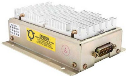
AA23 Speaker amplifier for driving either an eight (8) ohm speaker network or an array of headsets at a 100% duty cycle. Features muted or partially-muted outputs, adjustable gain and dual PTT key logic in/outputs.
