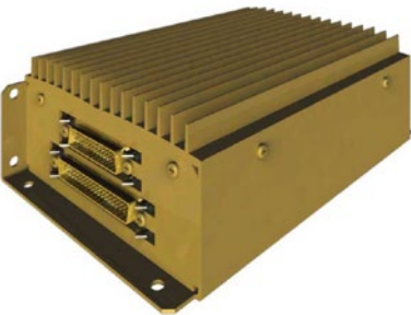
251 Paging/passenger speaker amplifier with 60-watt paging/stereo for helicopters and business class A/C. Can drive 1 ohm (4 x 4 ohm in parallel).
