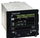
RT-7000PMR Combined Panel Mount, Multi-transceiver and User Interface Display
